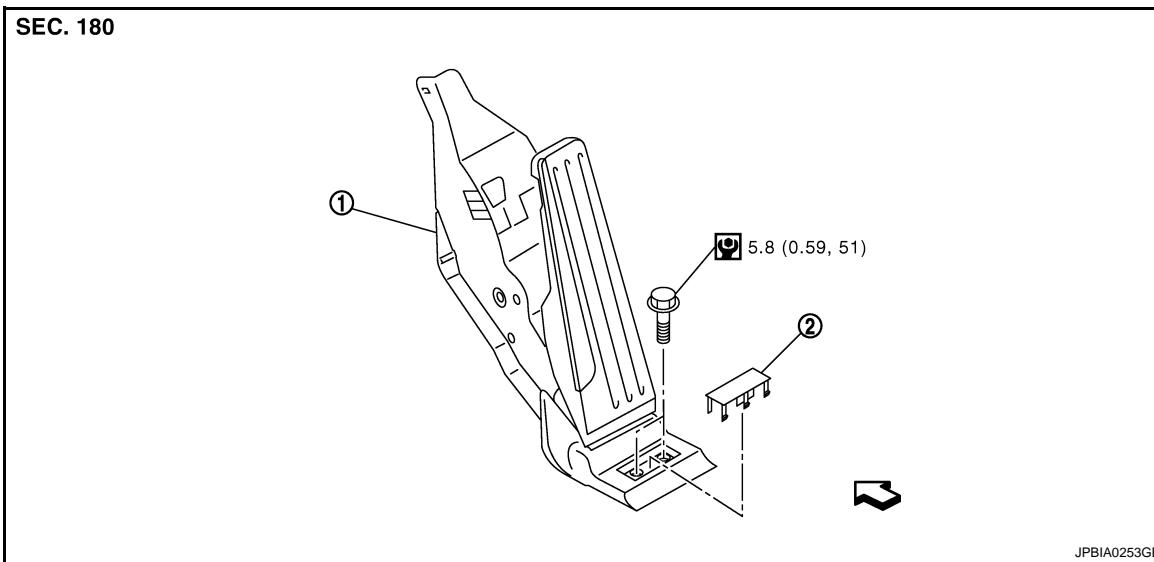
1. Accelerator pedal assembly      2. Bolt cap
